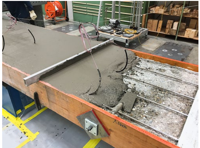
Versterking in reprofileermortel
